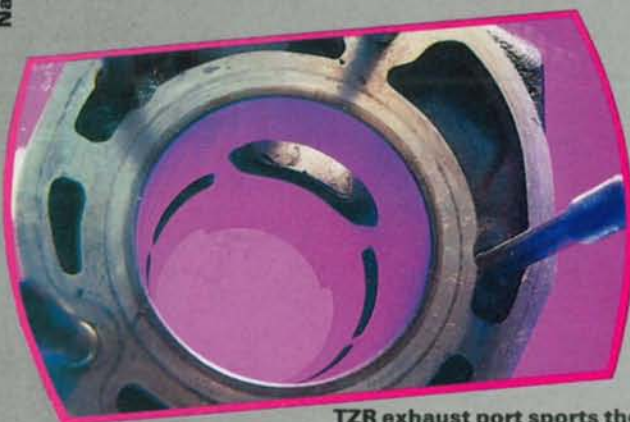
TZR exhaust port sports the most radical timing, but last generation's inlet and transfers can't keep up
