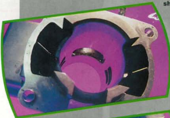
Exquisitely-crafted KR-1 is less coy; thingummy next to clutch basket is balance shaft, which bolts under bottom case
