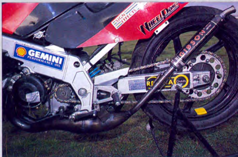
Peter Gibson's hydraulically formed chambers work as well on a stock bike as on the Supersport racer (see graph on opposite page).
